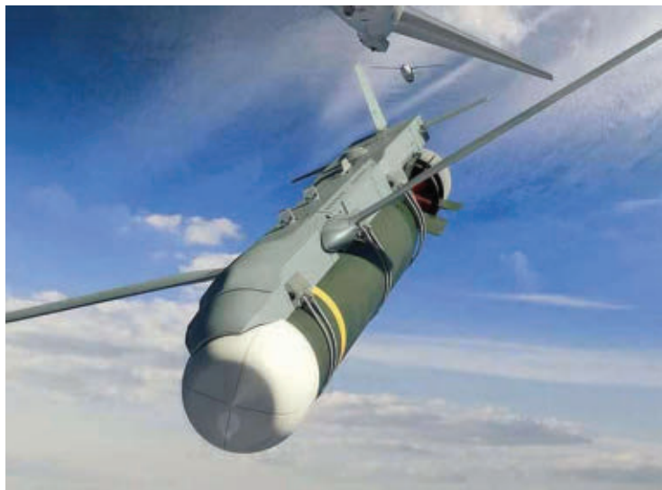
The Boeing High Altitude Anti-Submarine Warfare (ASW) Weapon Capability (HAAWC) jettisons its wings and tail as it enters the water and takes on its original role as a smart torpedo.
