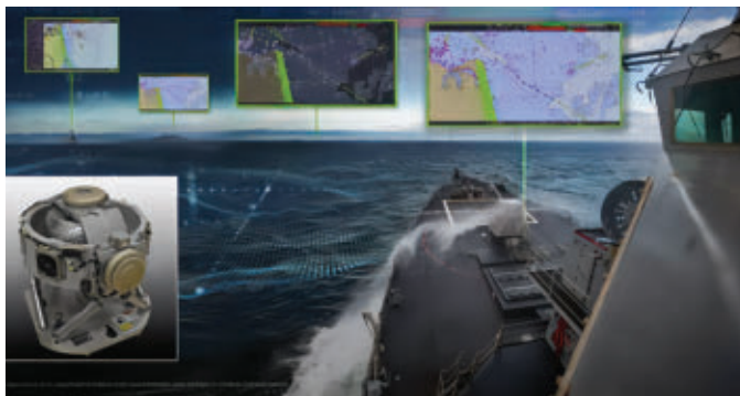
The Navy's Northrop Grumman AN/WSN-12 maritime navigation system uses the latest fiber-optic gyro (FOG) technology to provide fast and reliable navigation where satellite signals are unavailable.
