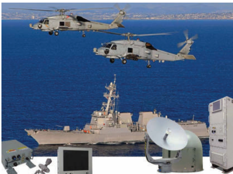
The AN/SRQ-4 Hawklink terminal provides Navy Arleigh Burke-class destroyers and Ticonderoga-class cruisers with command and control, and sensor data transfer.
