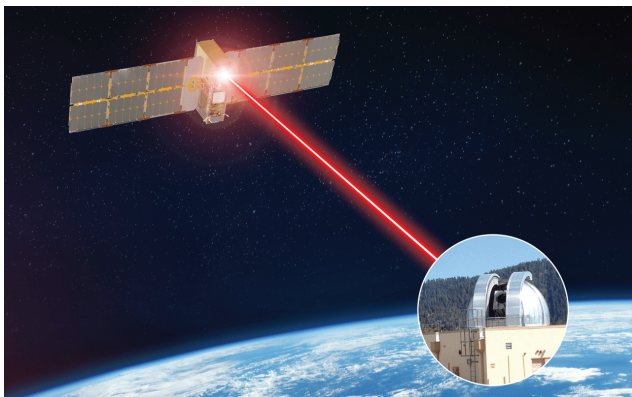
The NASA TeraByte InfraRed Delivery (TBIRD) optical communications payload, launched last year, showcases 200-gigabit-per-second data downlinks - the highest optical rate ever achieved by NASA.
