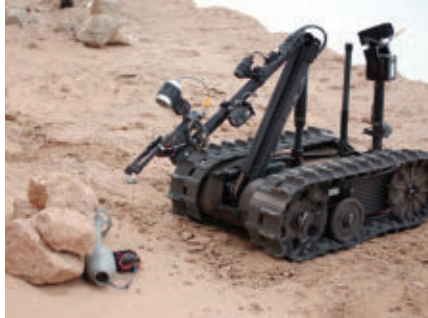
The U.S. Navy is using the QinetiQ MK 2 Man Transportable Robotic System (MTRS) for detecting and disposing of roadside bombs.
