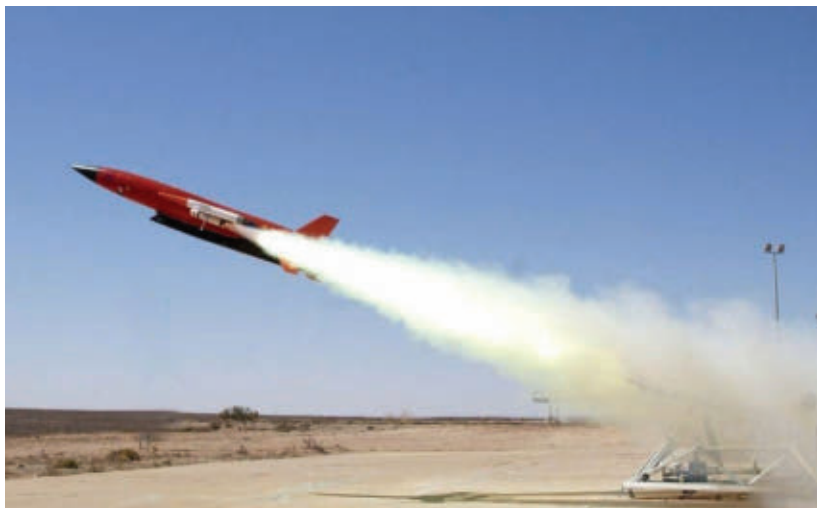
The Kratos BQM-177A unmanned target drone helps Navy surface warship crews practice how to evade and defeat enemy anti-ship missiles.
